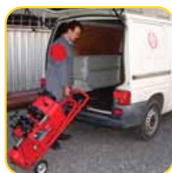
Position the upper part of the trolley on the vehicle entrance
