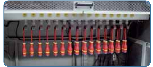
ALL INSULATED SCREWDRIVERS ARE TESTED AT THE END OF PRODUCTION THROUGH A GALVANIC BATH AT 10.000V
