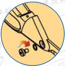
BLADE FRICTION ADJUSTABLE BY SCREW
