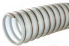
Flexible hose, light weight. Suitable for use as a cleaning/suction hose and to transport abrasive material such as wood shavings, sawdust, cement dust, granulates and technical gases in the chemical and petrochemical industries. Very good resistance to wear and ageing. Good resistance to fuels, oils, solvents and grease.
