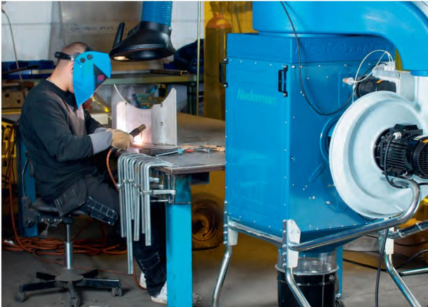
Complete mobile FilterBox unit with Original extraction arm.
