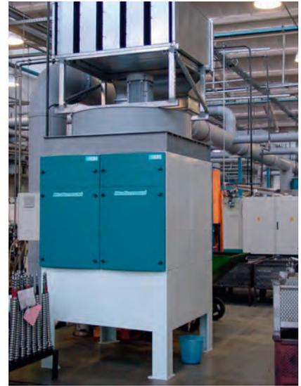
1. The contaminated air from the process is drawn into the lower chamber.
