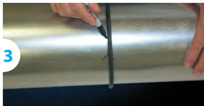
3 Use the enclosed rubber ring and mark the cutting point.
