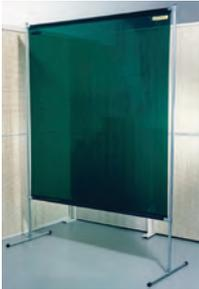
The protective curtain screens are easily movable for welding, grinding, turning, milling etc., and are ideal for the screening of temporary or permanent work places. The frame is manufactured from galvanised tube and the curtain of self-extinguishing PVC material (as the standard curtains above) and complying with EN 1598 for welding. Delivered complete with frame and curtain with total dimensions WxH=2000 x 2000 mm (just curtain H=1700 mm). Weight 7.5 kg.
