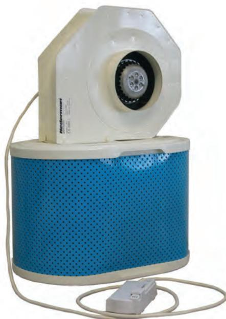
The unit consists of a separate filter cartridge and a N3 fan. It is designed for extraction and filtration of fumes and vapours emitted when soldering, gluing or working with solvents. For use in different combinations with the FX arms or the down flow grille FD 23.
