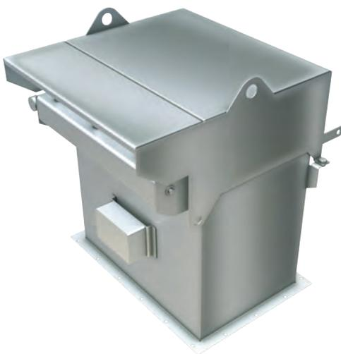
A compressed air cleaned cartridge filter with 24 m<sup>2</sup> filter surface, used for silo ventilation. Also available with a 2.2 kW fan (SiloSafe 24F). Strong welded construction in 4 mm heat-galvanised steel sheet. Filters can be replaced very easily as the hinged lid opens upwards and the cartridges are replaced from above. Needless to say, the filter is available in ATEX versions St1-St3.
