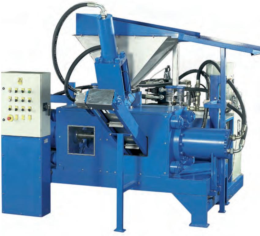
**A briquetter will reduce the volume of the material to enable savings in handling and transportation.**
