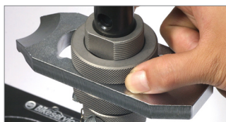
Adjusting the gear according to the size of spring coil.
